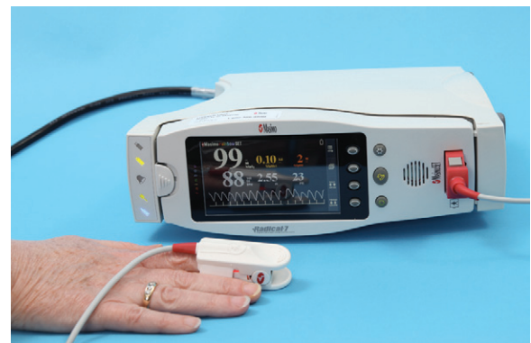
FIG. 3-11 Pulse oximeter shown with a clip and tape sensor probe. (From Potter et al., 2013.)
